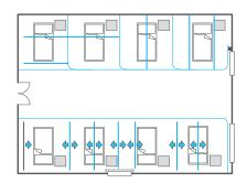
IV400 lends itself to many configurations within a hospital bed cubicle. The most common configurations of fixed track are shown here, but the specifier should take account of medical factors such as levels of usage, and the possible need of secondary IV provision at the foot of the bed.
