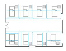
There are several alternatives for IV200 track positions. The most commonly used layout is a track parallel to the back wall and 1m out from it. A continous track is then possible over the line of beds, assuming an unobstructed ceiling. A second track may be positioned across the foot of the beds if required. Another alternative is a track running parallel to the bed. This gives IV provision at both the head and the foot of the bed, and also allows stacking of carriers against a wall.
